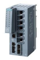
SCALANCE XC206-2SFP G (E/IP) managed Layer 2 IE switch; IEC 62443-4-2 certified; 6x 10/100/1000 Mbps RJ45 ports; 2x 1000 Mbps SFP; 1x console port; diagnostics LED; redundant power supply; temp. range -40 °C to +70 °C; mounting: DIN rail/S7 mounting rail/wall; redundancy functions; Office features (RSTP, VLAN,...); PROFINET IO device; Ethernet/IP-compliant; C-plug slot; Default EtherNet/IP
